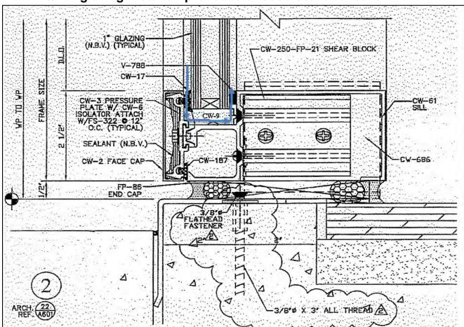
15/16" glazing installed produces a loose seal and leaks
