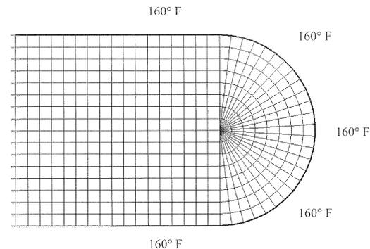
**2D Finite Element Model of EIFS bull-nose Specimen:** Model is subjected to a uniform thermal load of 160 F. Elements are 4 node quadrilaterals and are assigned the
