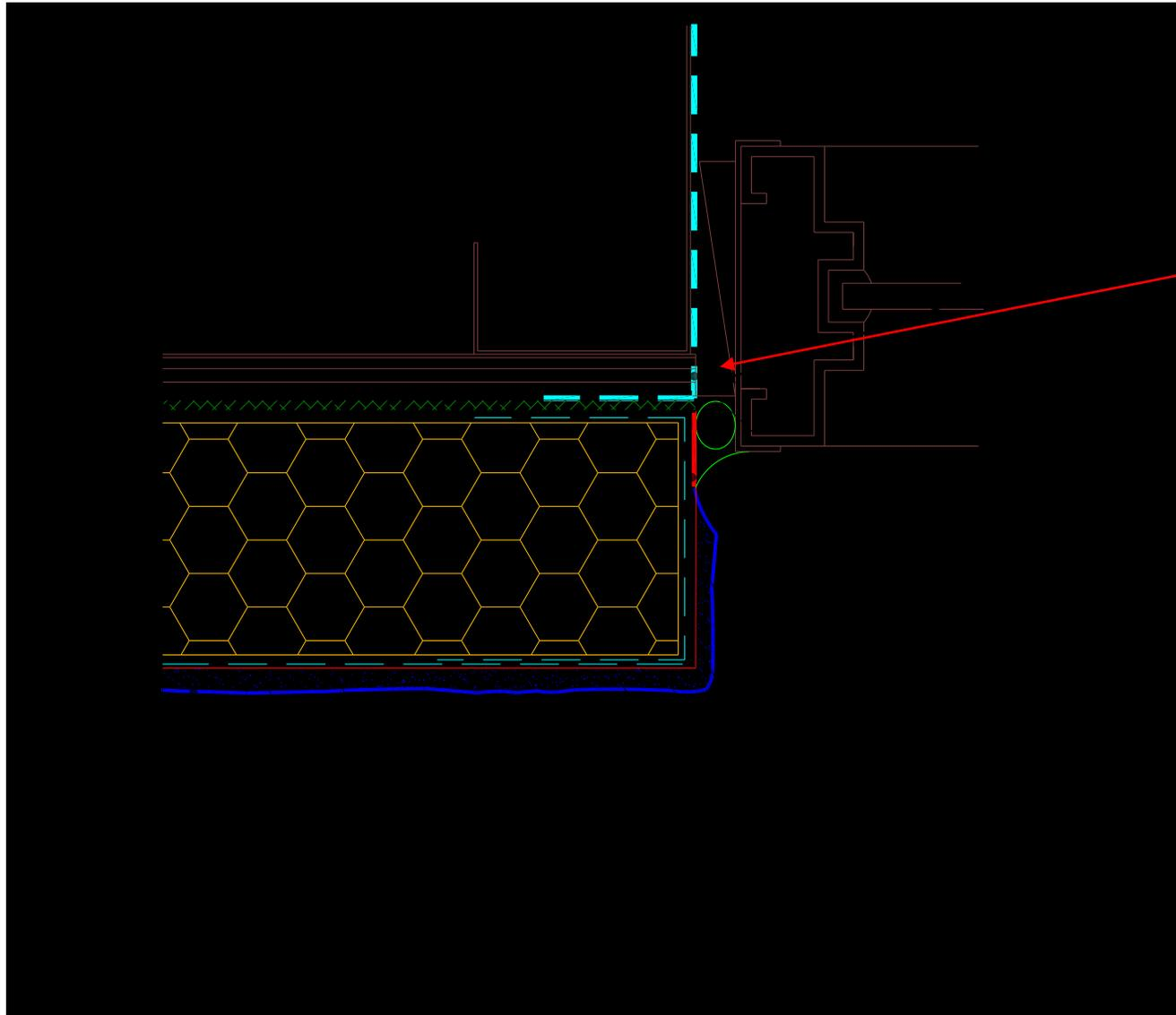
Manufacturer's standard detail is missing secondary seal to water resistive barrier.
