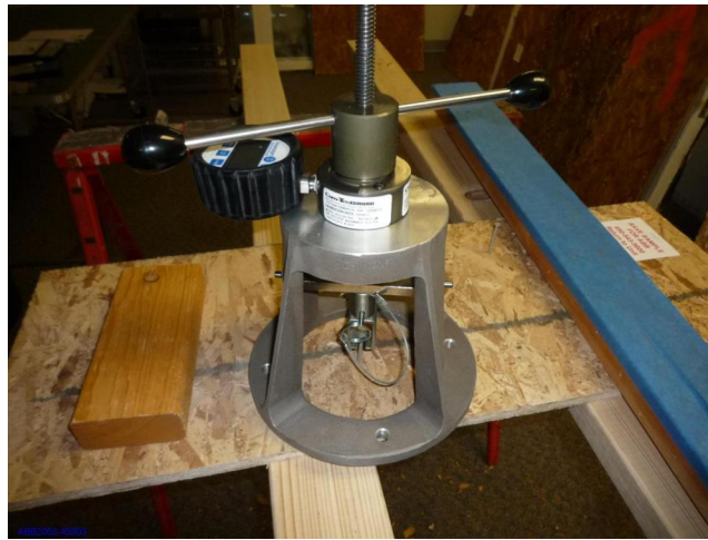
Figure 6C: ASTM D-1037 Nail Pull Tests – Loss of Strength
