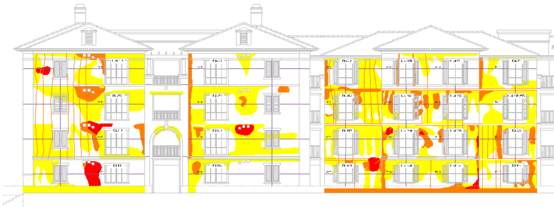
Figure 6A: Damage – South Elevation – Partial
