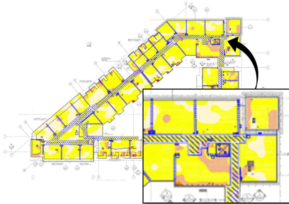
Figure 6: Nuclear Density Gauge Roof Survey Results
