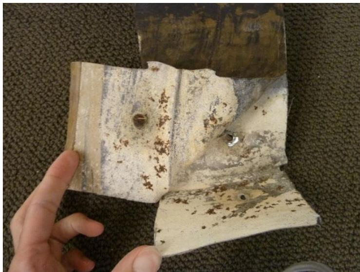
Figure 17: Corrosion of galvanized sheet metal flashings under 90 mils of fluid applied membrane
