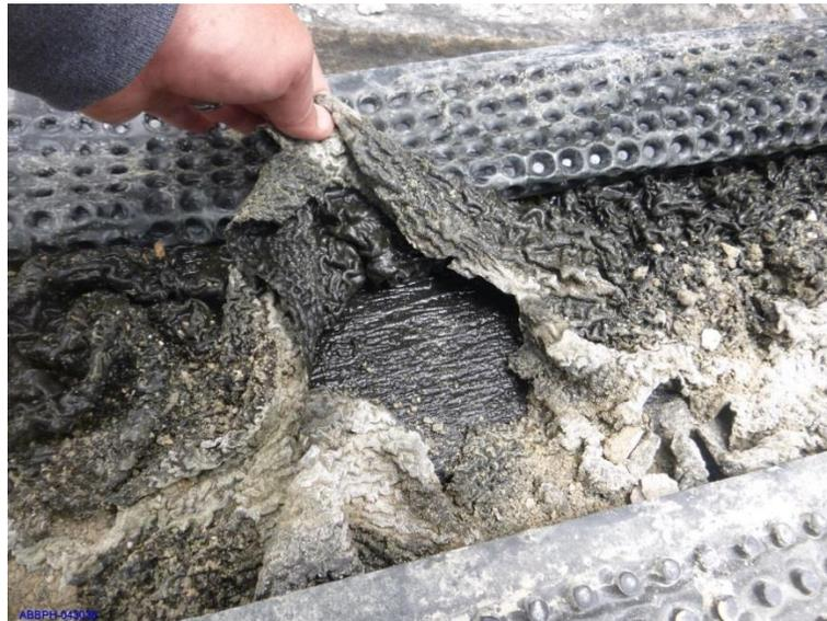
Figure 24: Modified polyurethane membrane is swollen and looks like the texture of “brain” or brainiac. Prolonged immersion of the membrane results in swelling and water absorption far beyond manufacturer’s published results.
