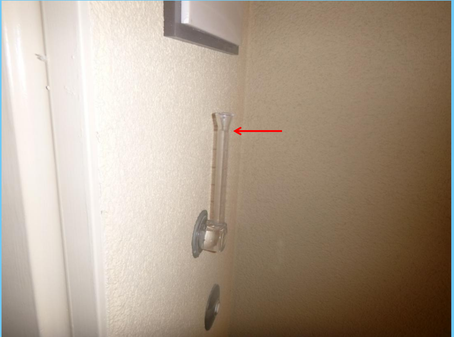
Building Pines B-1 Bldg. 1 Unit 1111 Rilem test over new Sto Finish-Tube is full at end of test.
