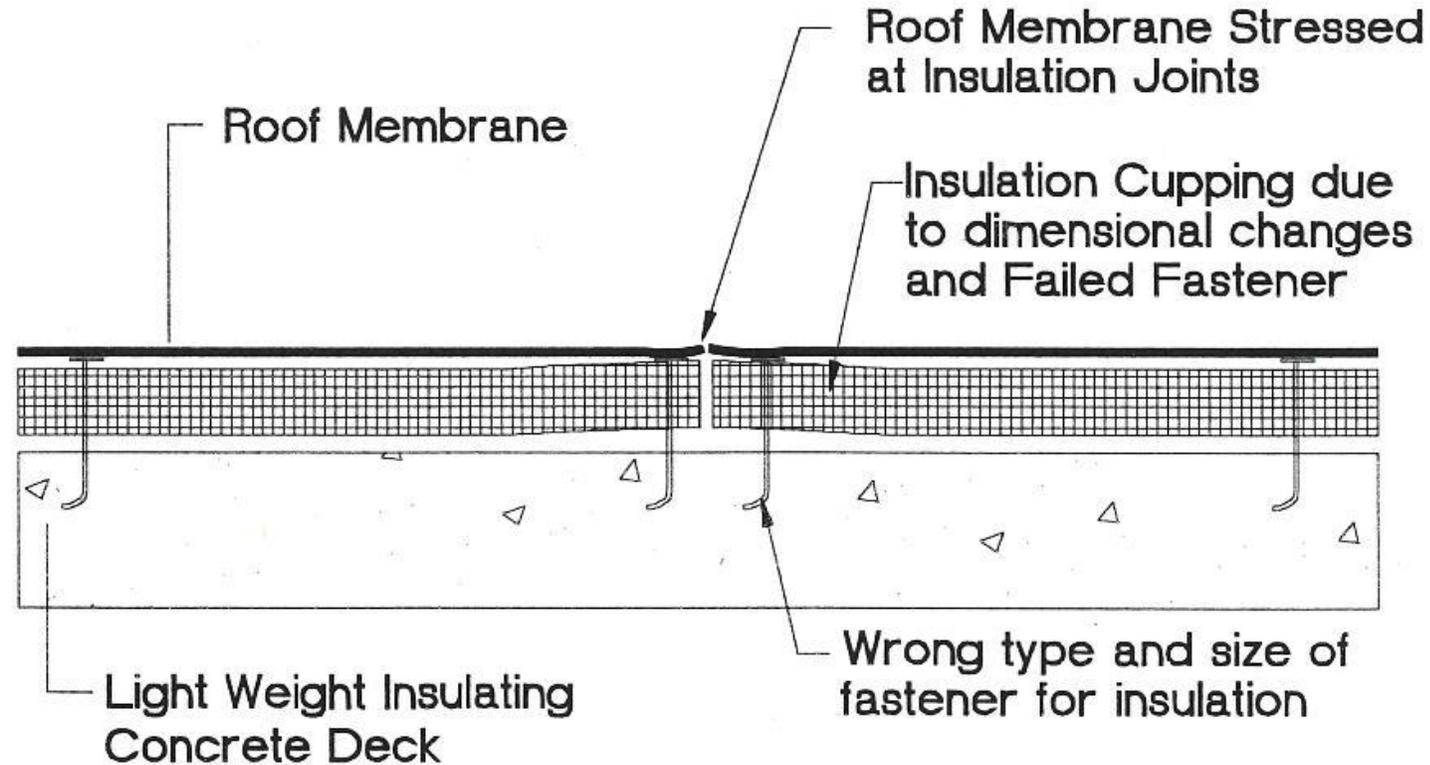
PICTURE FRAMING + ROOF SPLITTING CAUSED BY POOR FASTENING OF INSULATION BOARD TO SUBSTRATE
