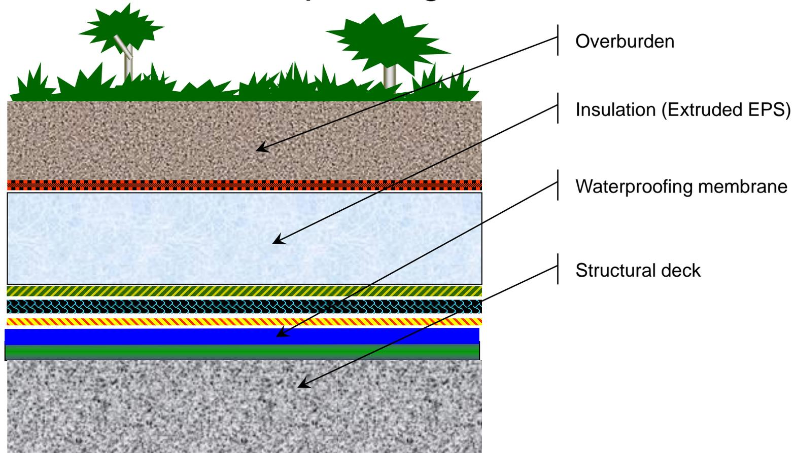
Insulation must have sufficient compressive strength (60 to 100) psi and must not absorb water
