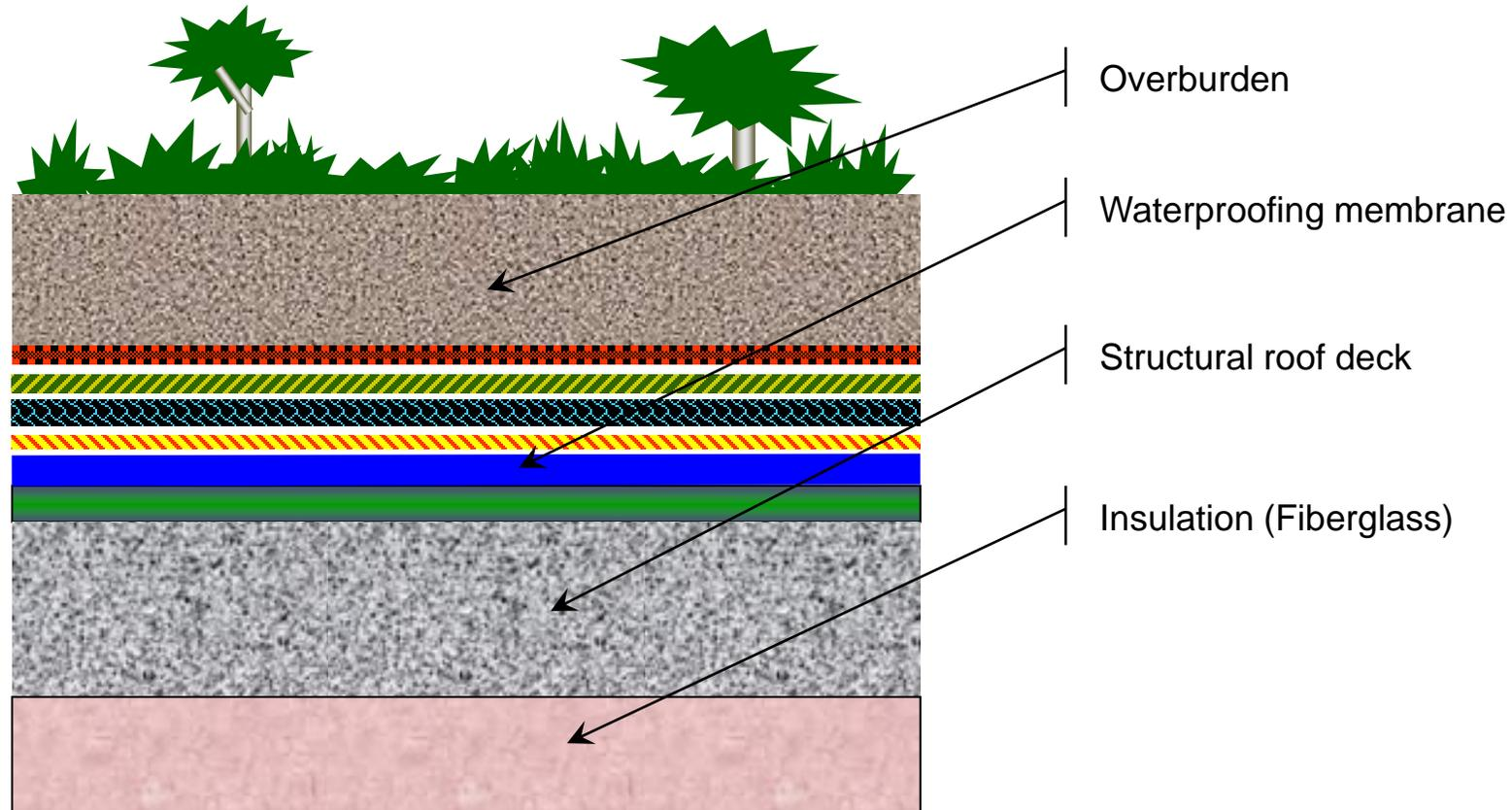
Insulation is independent of waterproofing and roof garden
