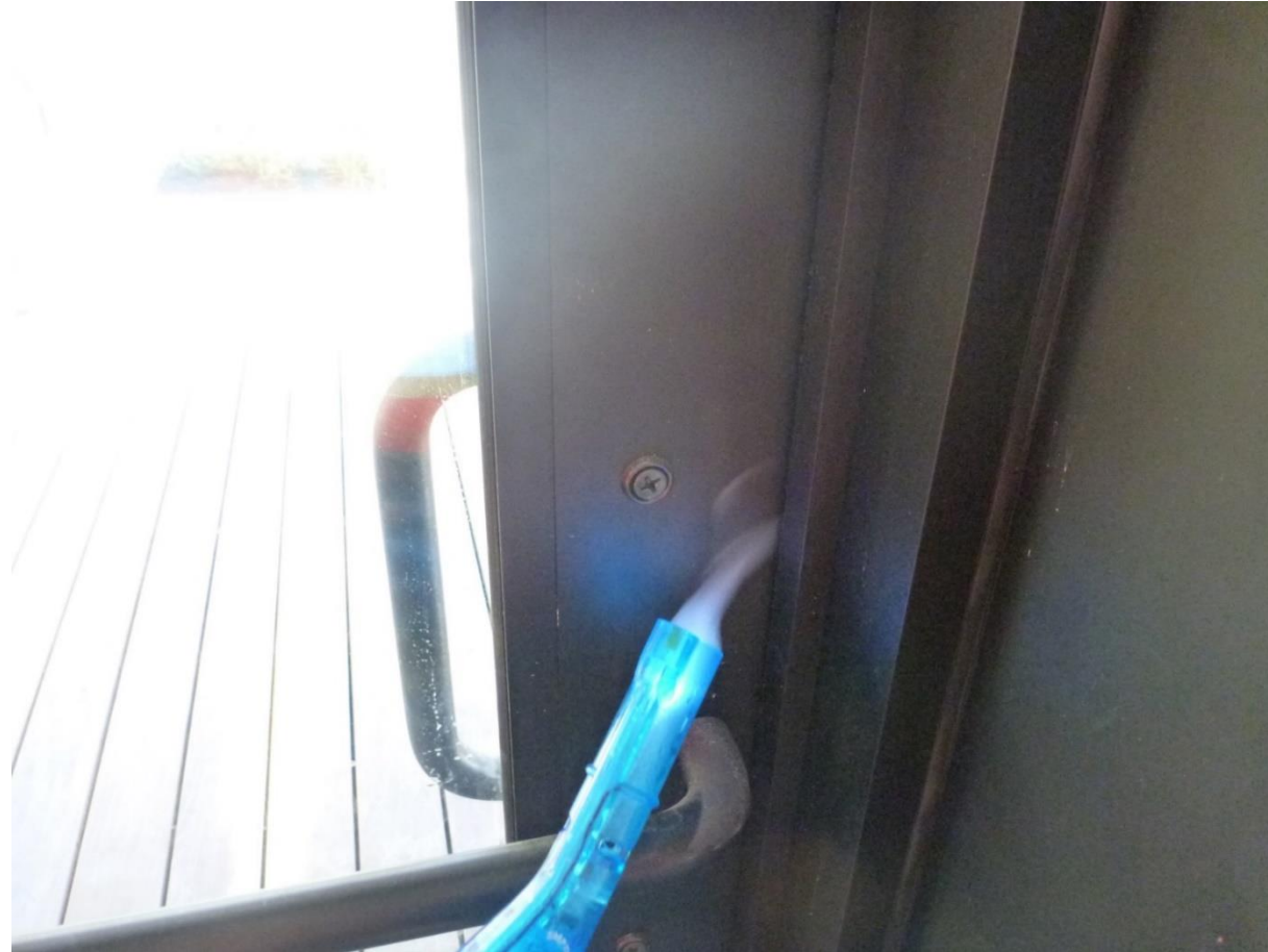
Air leakage identified by tracer testing
