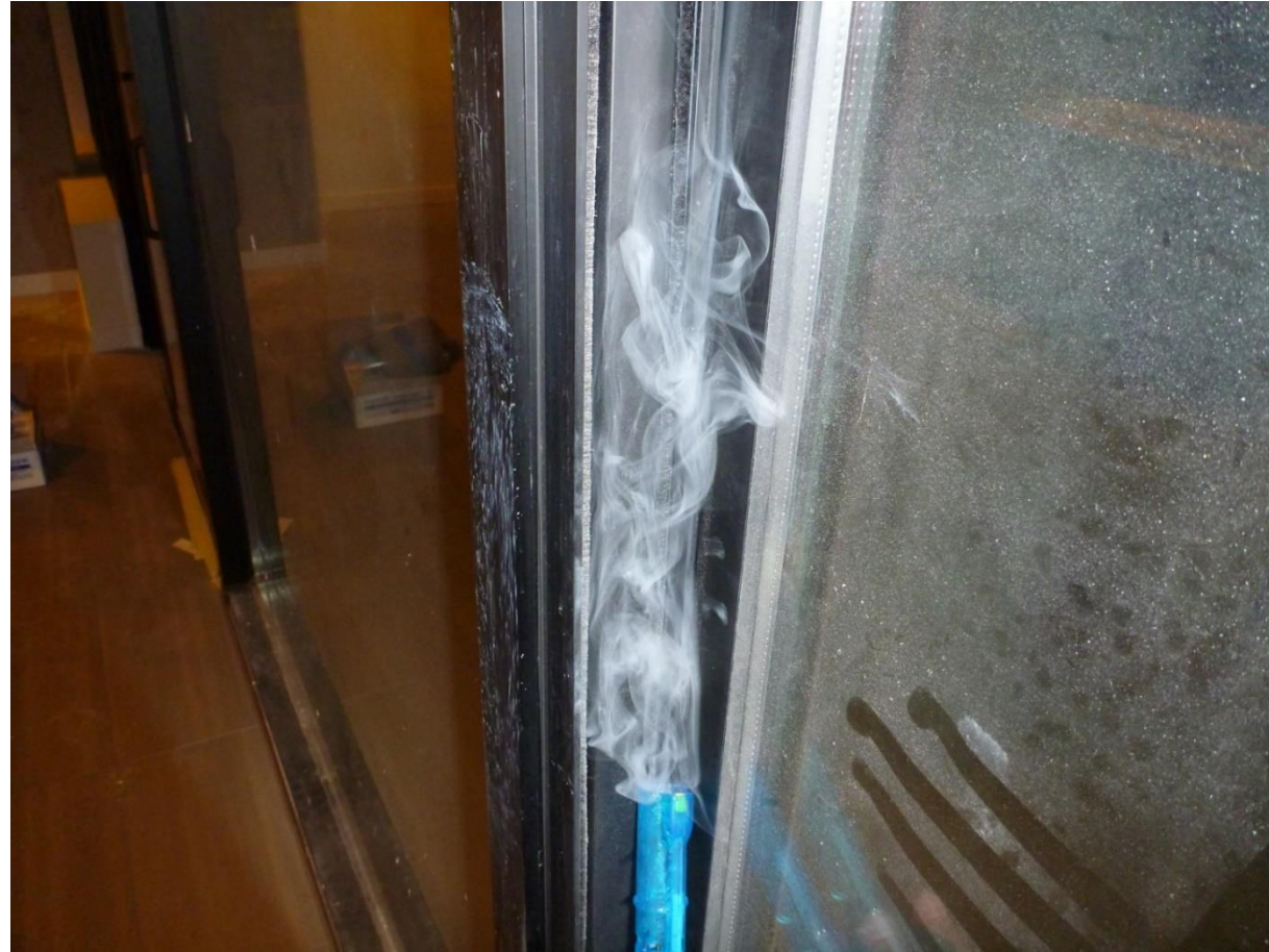
Tracer smoke test, no leakage
