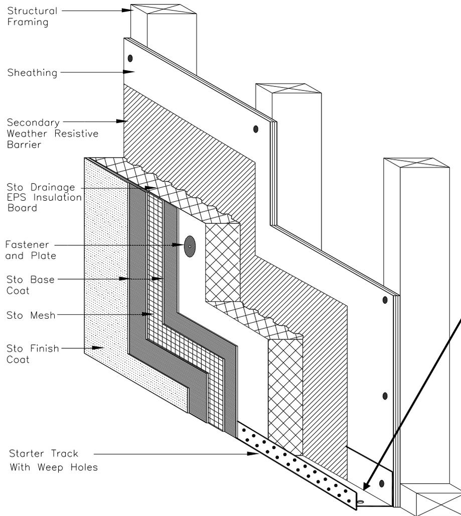
Unless system is tested as a “Barrier System” it must have weather resistive barrier and weep mechanism
