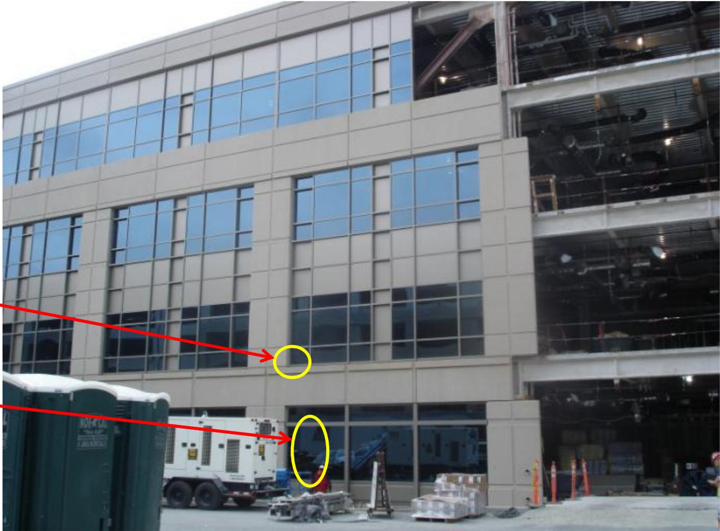
Leak observed on the 2<sup>nd</sup> floor after the first spray test at the GFRC panel
