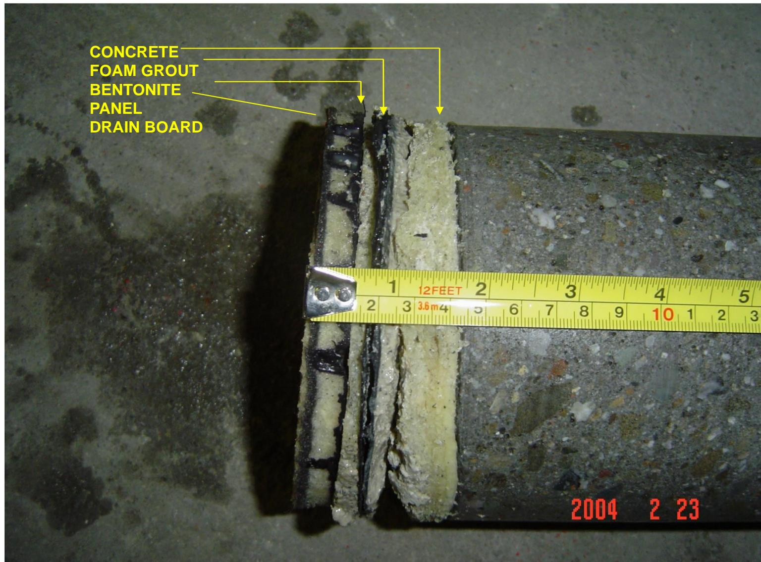
Voids were present on both sides of the retaining wall and ranged from 1" thick to up to 4" thick. Grout in post-repair picture shows measurable void.
