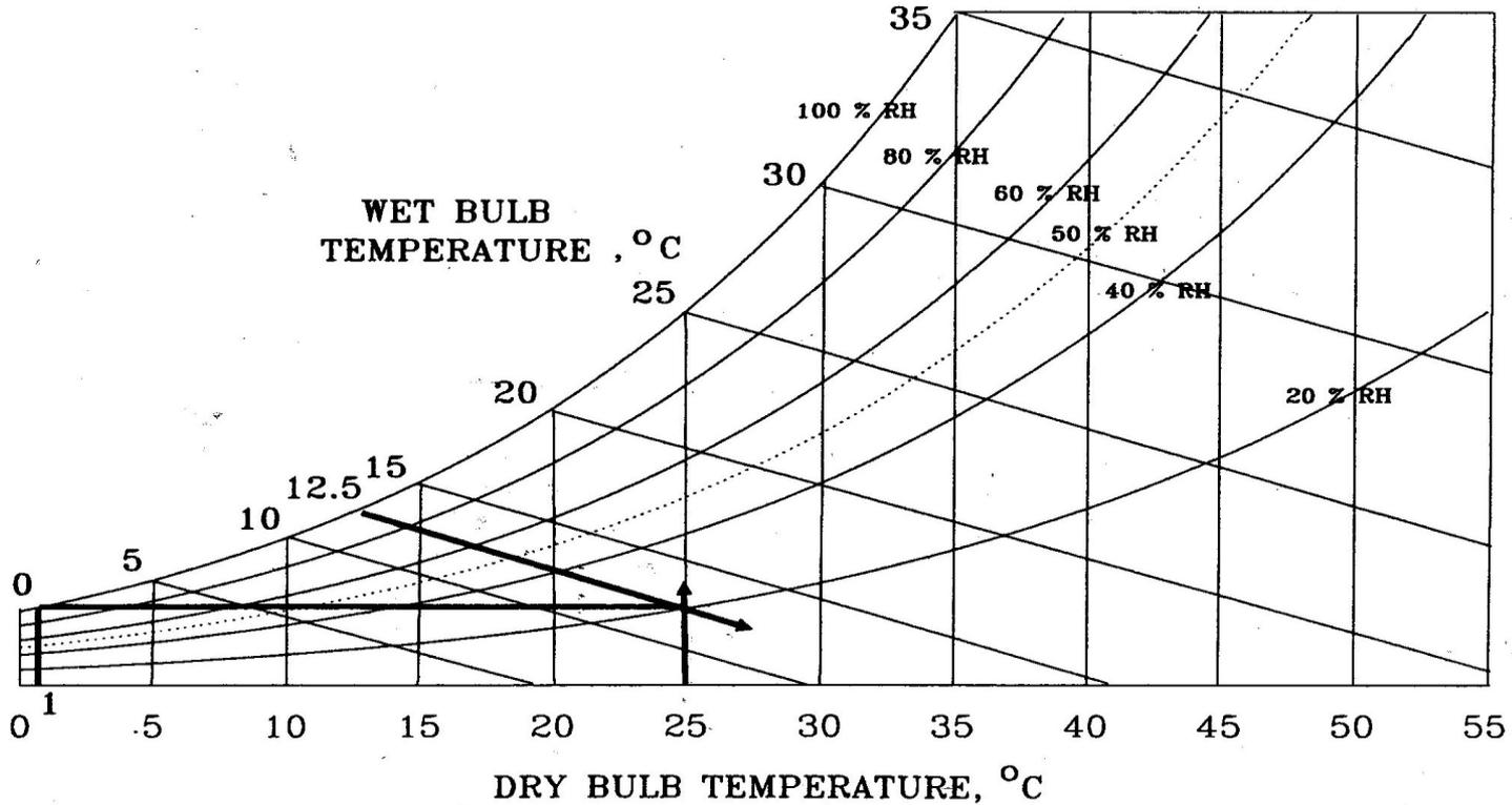
FIG. A4—Calculation of relative humidity and dew point temperature from psychrometric measurements.
