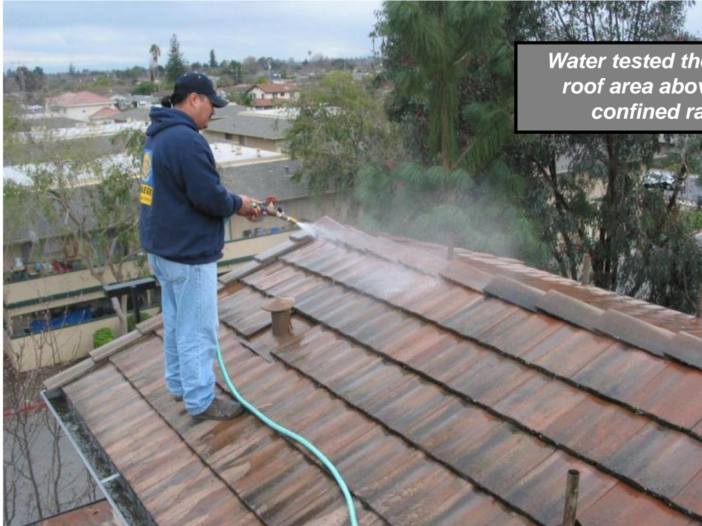
*Water tested the gable roof area above the confined rake*
